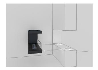
Fix it to the floor using the supplied screws through the holes in the bottom of the fireplace (after installing the pins).
